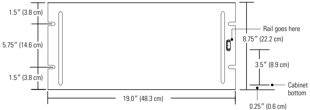
Figure 17. RBC-3 Front Panel Bolt Slot Measurements
